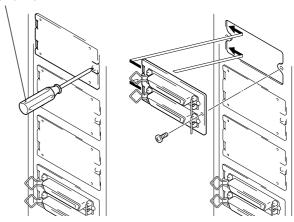
Place the drive on the changer guide rails, push the drive in until the lock lever on the drive shifts to the locked position. Maybe you can hear a clicking sound then.
